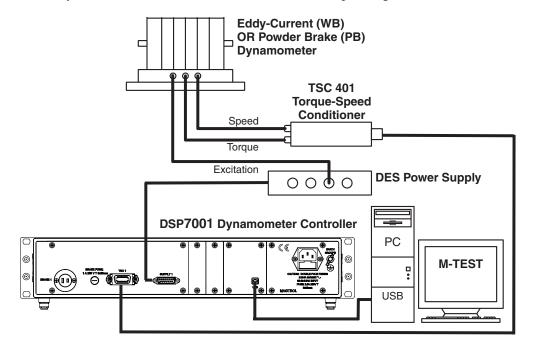
Figure 4–2 PC-Based Test Configuration with M-TEST Software
