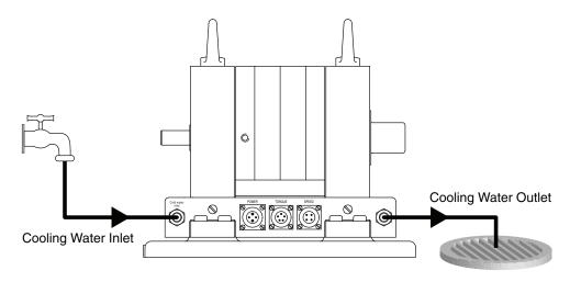
Figure 3–1 Open-circuit Cooling Example
