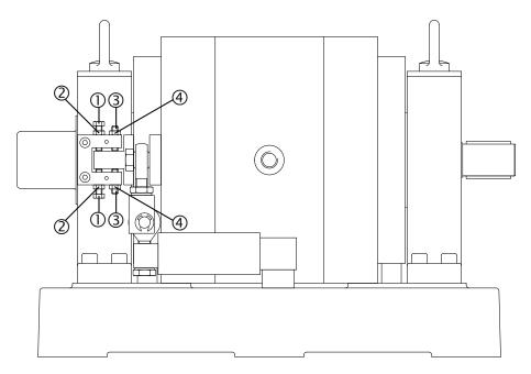
Figure 2–4 WB/PB 115 Load Cell Locking System
