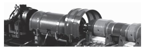
Figure 2–7 Example of Protective System
