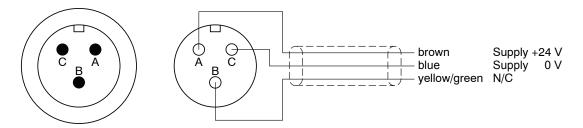
Figure 4-6 Control Signal Cable for WB/PB 65, 115 and 15 Tandem Dynamometer Clutches
