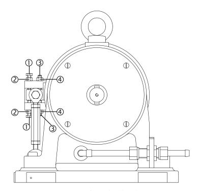
Figure 2–3 WB/PB 65 Load Cell Locking System
