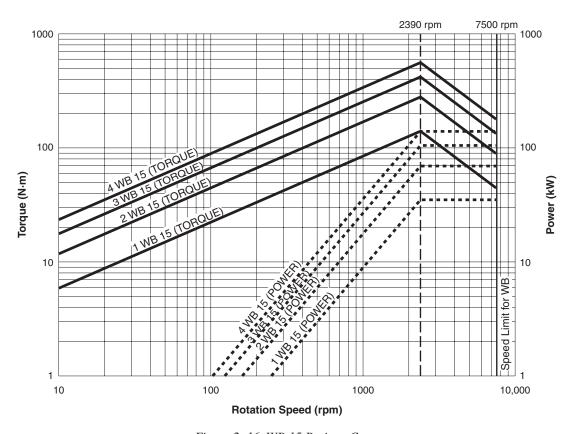
Figure 2–16 WB 15 Ratings Curve
