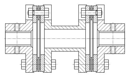
Figure 2–6 Couplings Using Key Clamping
