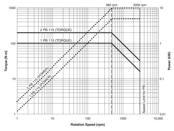
Figure 2–15 PB 115 Ratings Curve
