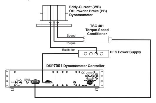
Figure 4-1 Manual Test Configuration
