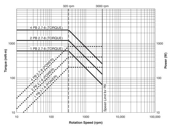
Figure 2–9 PB 2.7 Ratings Curve
