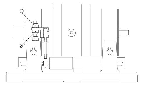
Figure 6–2 WB/PB 43 Overload Protection Calibration
