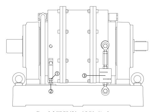
Figure 2-5 WB/PB 15 Load Cell Locking System
