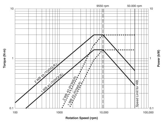
Figure 2–10 WB 43 Ratings Curve
