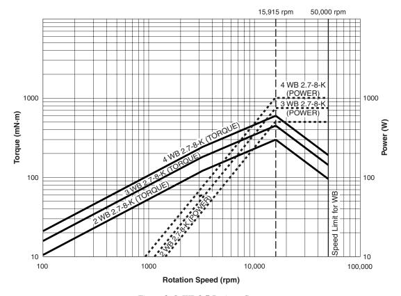
Figure 2–8 WB 2.7 Ratings Curve
