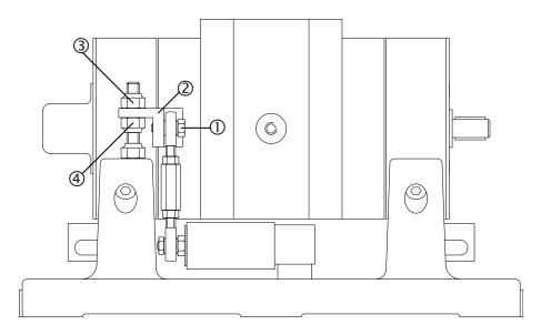
Figure 2–2 WB/PB 43 Load Cell Locking System
