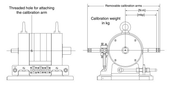
Figure 6–1 Calibration Arm Mounting
