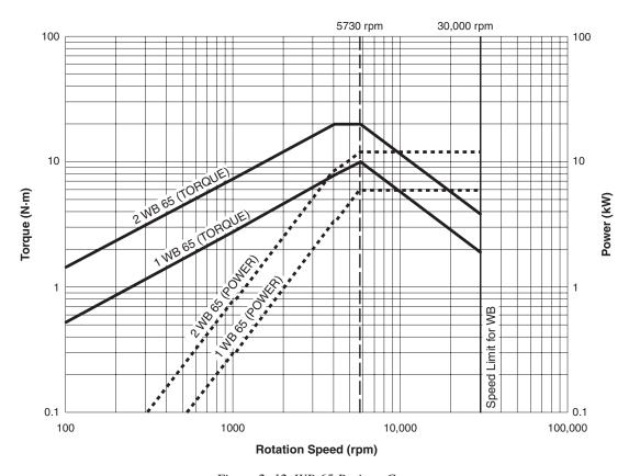
Figure 2–12 WB 65 Ratings Curve
