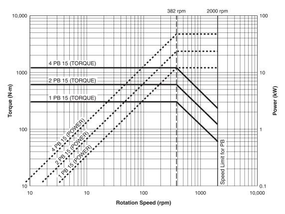
Figure 2–17 PB 15 Ratings Curve
