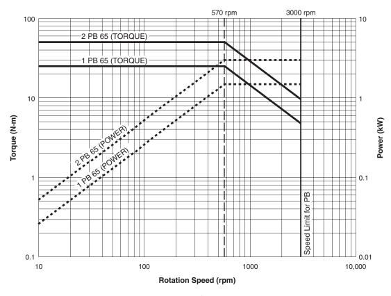
Figure 2–13 PB 65 Ratings Curve
