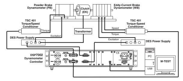
Figure 4–3 Tandem Configuration
