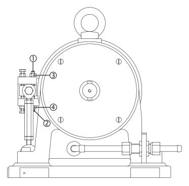
Figure 6–3 WB/PB 65 Overload Protection Calibration
