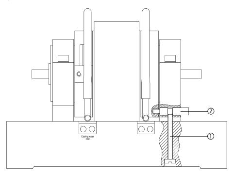
Figure 2-1 WB/PB 2.7 Load Cell Locking System
