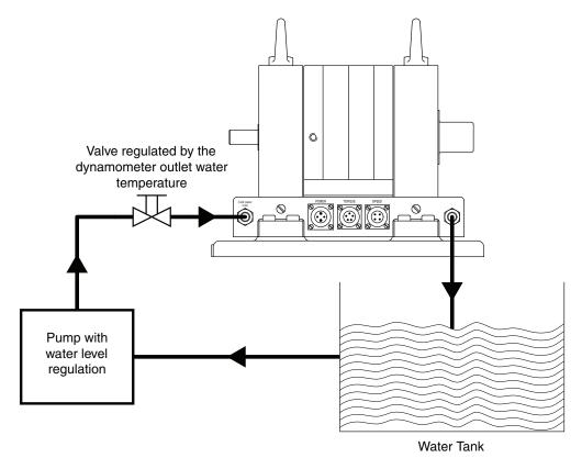
Figure 3–2 Closed-circuit Cooling Example
