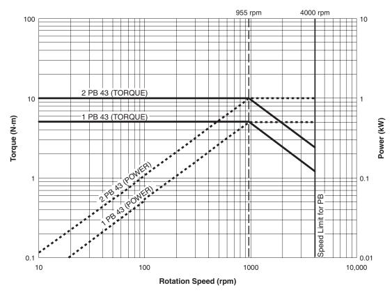
Figure 2–11 PB 43 Ratings Curve
