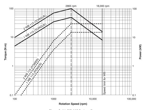
Figure 2–14 WB 115 Ratings Curve
