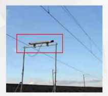
The small size of the OVHWizard allows a wide range of application in contact wire position detection.
