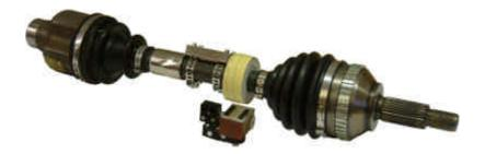
The IH2 pickup head is shown here supported by the universal mounting bracket and near to a shaftmounted loop made from the CAK kit components.
