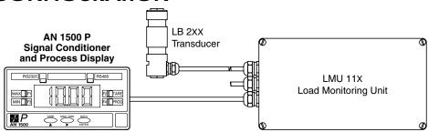
The AN 1500 P is used with Magtrol Load
