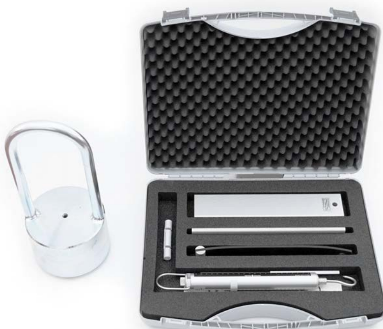
Case with measurement rods 1 to 5 with spring balance
