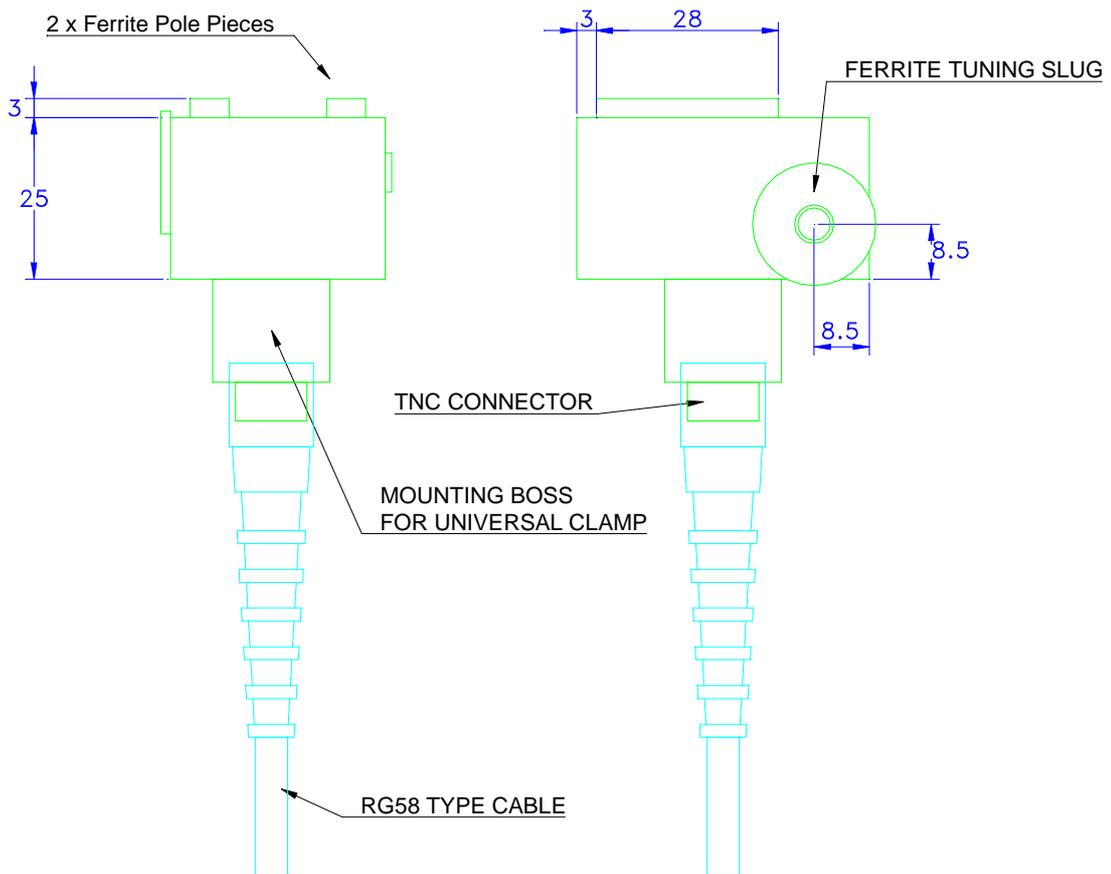
Figure 16 - Dimensioned Drawing of Inductive Head IH2
