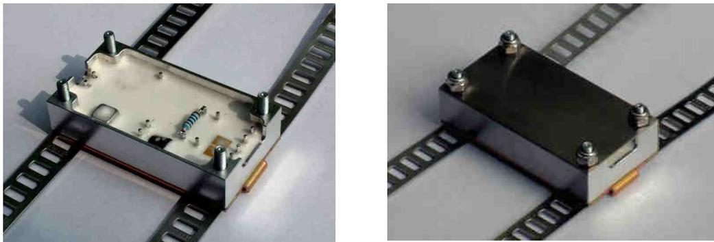
Figure 2 – TX31D with Strapping Plate and Mu Metal Cover
