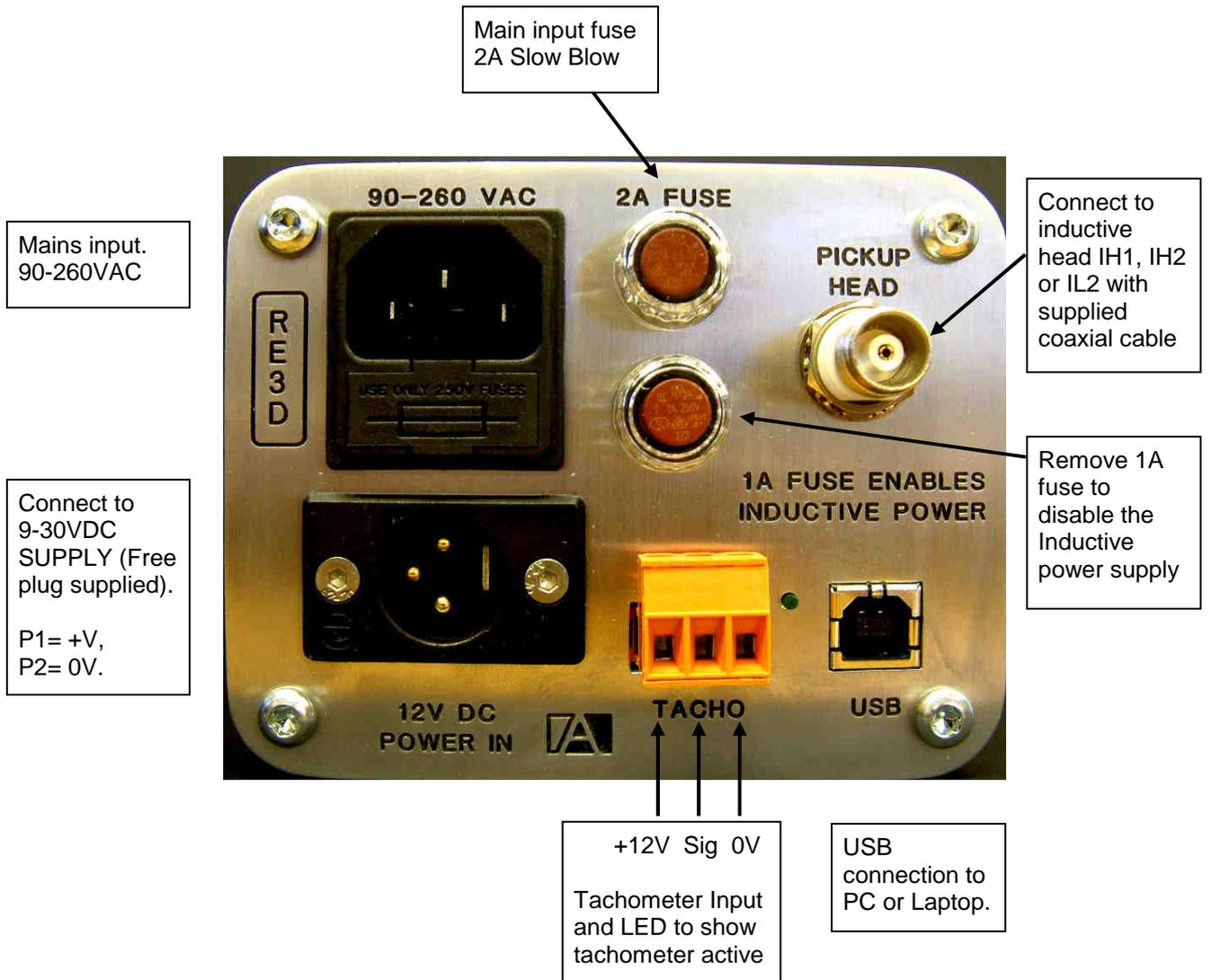
Figure 6 - Demodulator RE3D Controls & Connections
