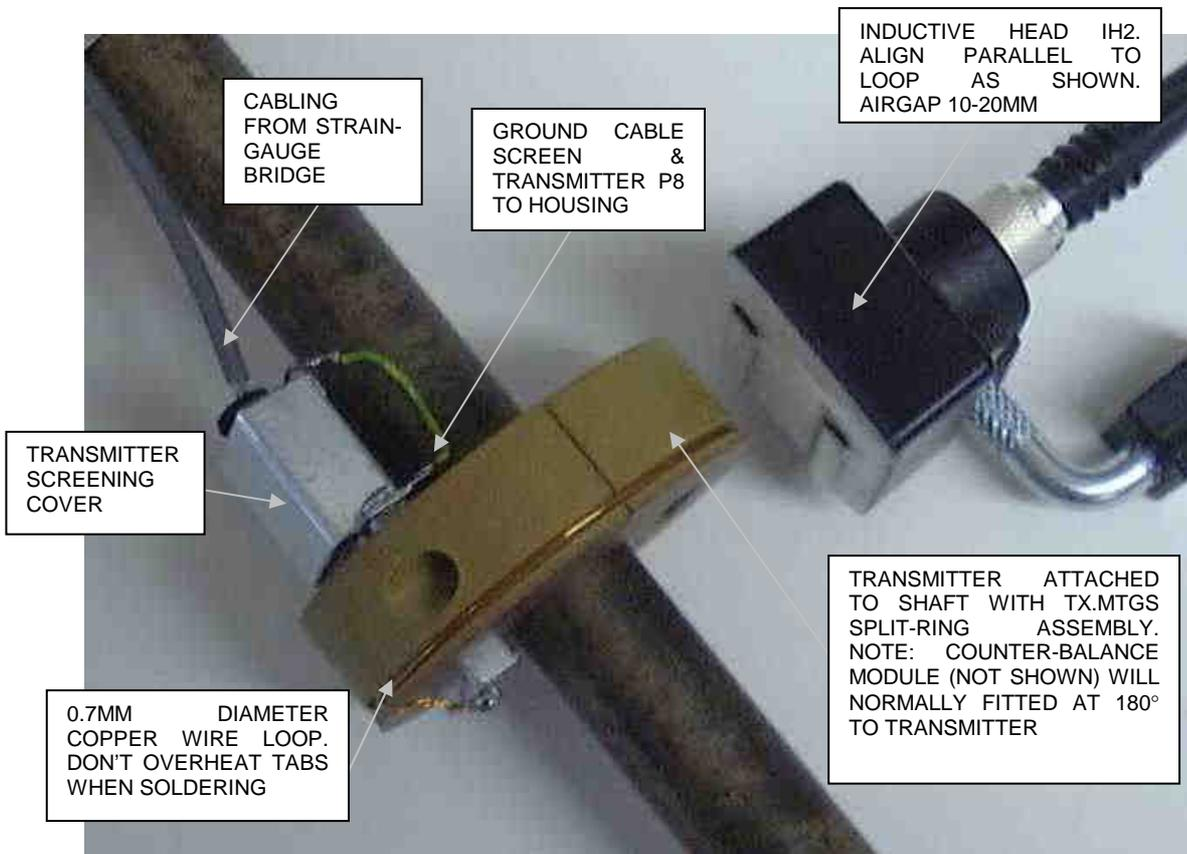
Figure 7 - Installation of Transmitter and Split-Ring "TX.MTGS" and Inductive Head IH2
