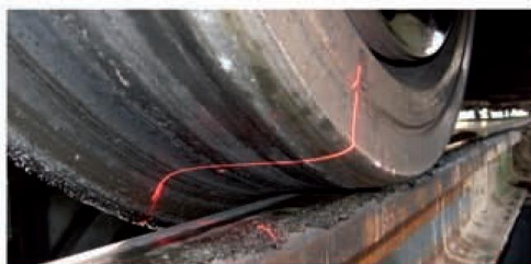
Contactless measurement Based on laser-camera triangulation
