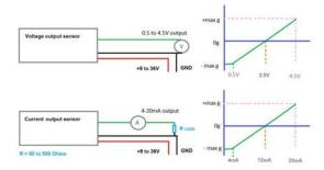
Notes: For the 4-20mA output version, the power supply requirement must deliver a minimum of 85mA.
