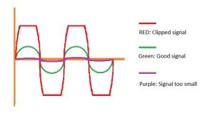
If you choose an accelerometer with a range that is too low, the output will reach the maximum and "clip" causing loss of data.
