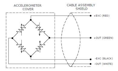
TE CONNECTIVITY SENSORS /// MODEL 1201 & 1201F ACCELEROMETERS
