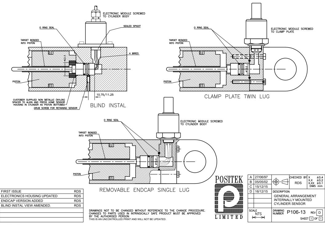
TARGET TUBE OPTION NOTES:-1. SPECIFY TUBE MATERIAL; CODE:-'R' STAINLESS STEEL 316 \( \phi 9.45.\)
