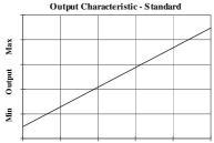
Retracted Linear Displacement Extended
