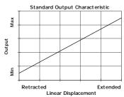
Output Characteristic: Target is extended 9 mm from end of body at start of normal travel. The output increases as the target extends from the sensor body, the calibrated stroke is between 5 mm and 800 mm.
