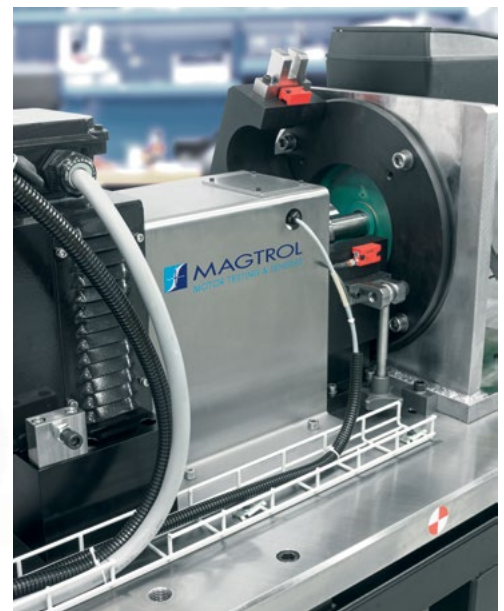
Fig.2-11 Test bench with fixed and movable metal guard with safety switch.
