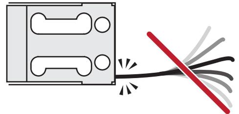
3. Properly secure sensor cable to limit cable movement influence.
