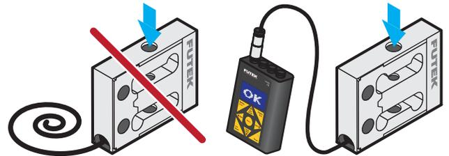
4. Install in a dry, clean environment, unless IP rating allows for other environments
