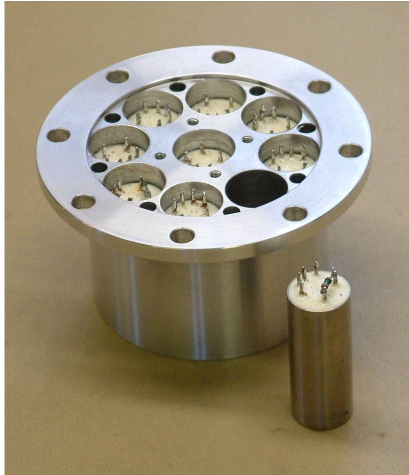
9 CHANNEL FREQUENCY MULTIPLEX TRANSMITTER ASSEMBLY FOR SHAFT BORE INSTALLATION IN GAS TURBINE COUPLING
