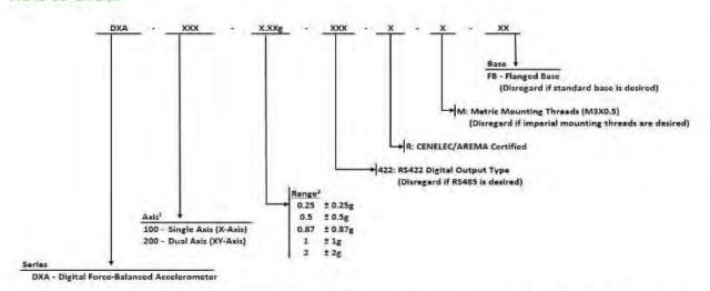
Example: DXA-100-0.25g-R = DXA series, single axis, ±0.25g range, RS485 output, CENELEC/AREMA certified, imperial mounting threads, standard base
