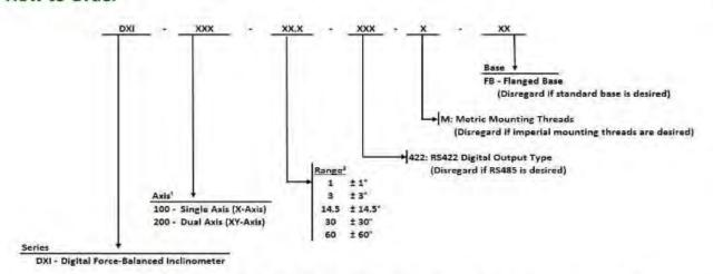
Example: DXI-100-14.5 = DXI series, single axis, ±14.5° range, RS485 output, imperial mounting threads, standard base
