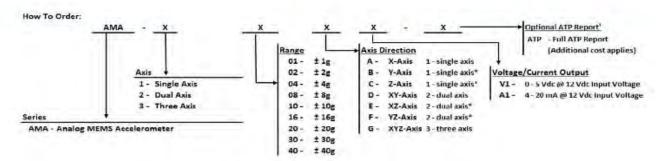
Example: AMA - 2 - 02 - D - V1 - ATP AMA Series, dual axis, ±2° range, XY-axis, 0 - 5 Vdc Output, Full ATP Report
