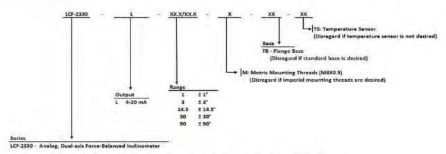
Example: LCF-2330-L-90/90 = LCF-2330, 4-20 mA output, ±90° range, imperial mounting threads, standard base
