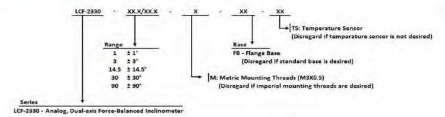
Example: LCF-2330-90/90 = LCF-2330, ±90° range, imperial mounting threads, standard base
