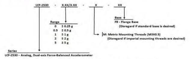
Example: LCF-2530-5/5 = LCF-2530, ±5 g range, imperial mounting threads, standard base
