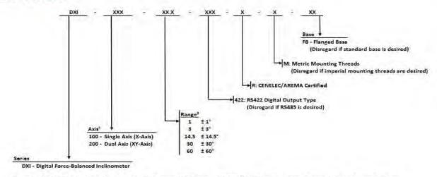
Example: DXI-100-14.5-R = DXI series, single axis, ±14.5° range, RS485 output, CENELEC/AREMA certified, imperial mounting threads, standard base
