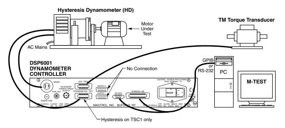
Figure 2–16 PC-Based System Configuration with Model DSP6001 Controller
