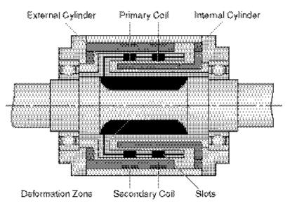
Figure 3–1 TM Torque Transducer Principal Elements
