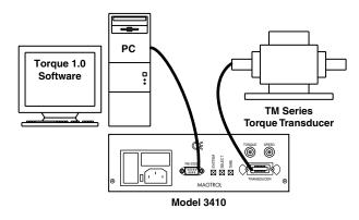
Figure 2–12 PC-Based System Configuration with Model 3410 Display
