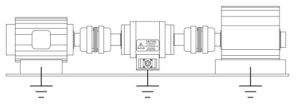
Figure 2–17 Common Grounding
