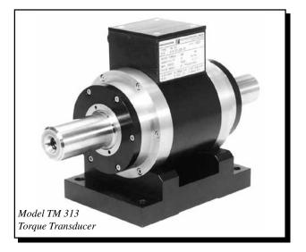
DC voltage, provides torque and speed signals without any additional amplifier. The transducer is a stand-alone measuring chain. Connections are made by means of a 6-pole male connector mounted on the housing. A removable aluminium base—delivered as standard with TM and TMHS models, and as an option for TMB transducers—allows fixed mounting of the transducer.
