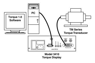
**PC-Based System Configuration** Torque Transducer with Model 3410 Display and Torque 1.0 Software
