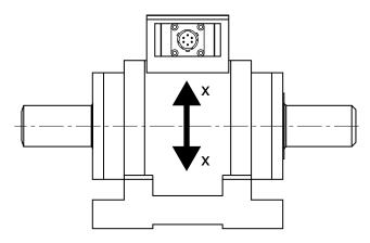
Figure 2–4 Radial Displacement
