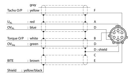
Figure 2-21 ER 107 Pin Configuration
