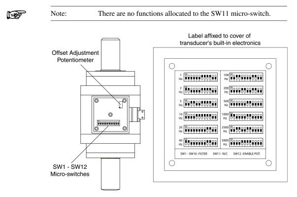
Figure 2–6 SW1 – SW12 Micro-switches and Offset Adjustment Potentiometer
