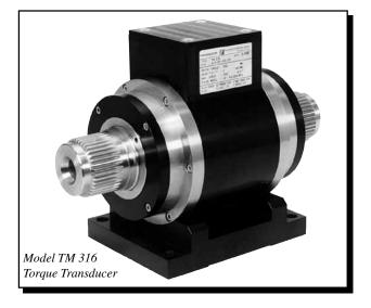
supplied by single DC voltage, provides torque and speed signals without any additional amplifier. The transducer is a stand-alone measuring chain. Connections are made by means of a 6-pole male connector mounted on the housing. A removable aluminium base, delivered as standard, allows fixed mounting of the transducer.
