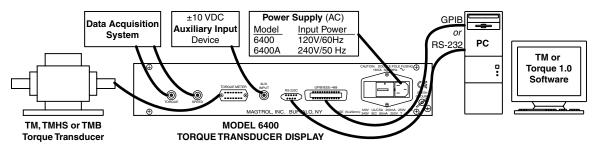
Figure 2–14 PC-Based System Configuration with Model 6400 Display
