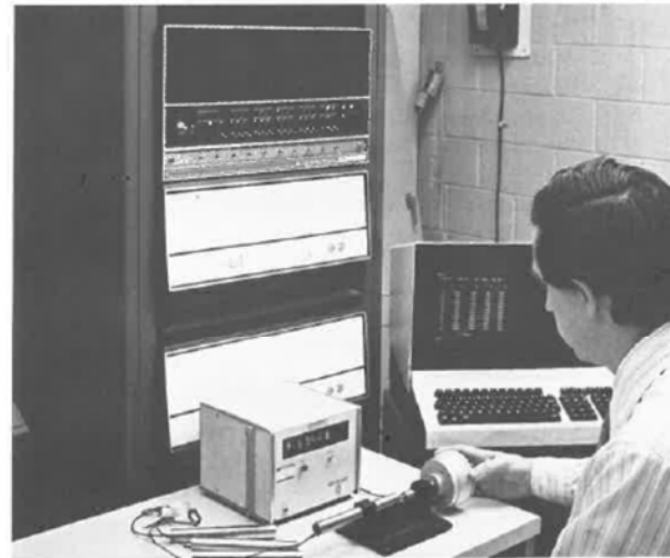
Fig. 14.2 On-line calibration equipment connected to mini-computer.
