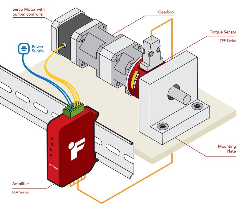
In certain applications, like managing constant tension while winding material onto a spool, it is necessary for the servo motor to generate a fixed amount of torque. Frictional loss and motor speed change necessitate the inclusion of a closed loop control system. To accomplish this, place a reaction torque sensor between the servo gearbox and its mounting location to measure the generated torque.
